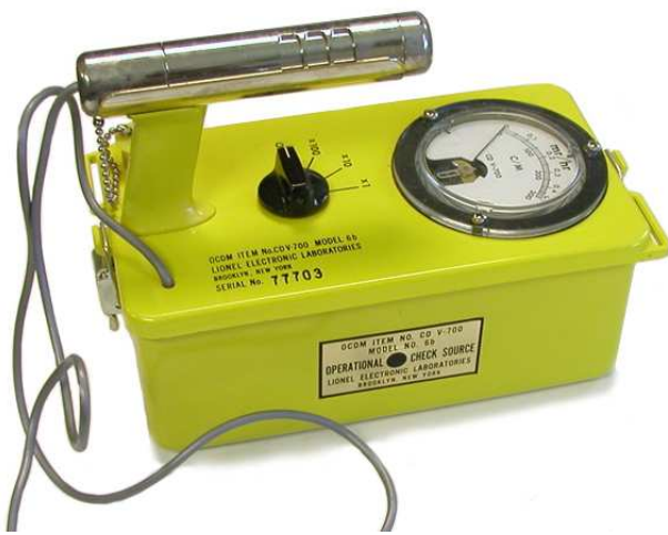
Fig. 13. Lionel Electronics Laboratories (LEL) was an ill-fated venture by The Lionel Corporation when it acquired Anton Electronics Laboratories a company that specialized in producing radiation detectors. Most of its sales were to the U.S. government. Its most successful product was the CDV-700 Geiger survey meter produced for the U.S. Office of Civil Defence. Very rugged and long-lasting, about 82,000 were made. Around 1965, Lionel closed LEL following recurring losses and possible mishandling of proceeds from sales.
